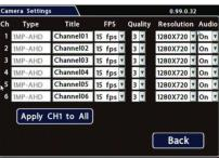
Set unused camera FPS speeds to Off, so the DVR will not generate video loss events.
